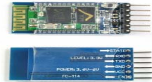
Fig 3: The HC05 Bluetooth module
